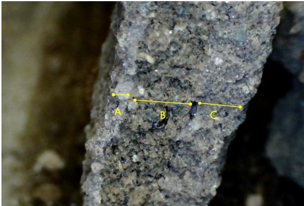
A: Likely a layer of the adobe brick that adhered to layer B, B: earliest layer of earthen plaster C: latest 'pink' layer of earthen plaster
